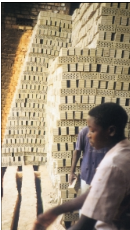
Fig. 2: Bricks stacked with a finger's width between them
